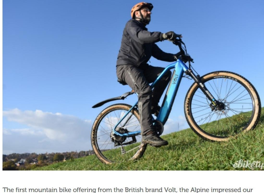
paired with a torque sensor. The 504Wh battery is removable and our 70kg tester managed 40 miles of off-road on one charge. If that's not enough, you can buy bigger batteries for more range. The front forks are Suntour X1 with 120mm travel which suggests this isn't something for particularly technical trails, but a fun ride on light off-road nonetheless.
